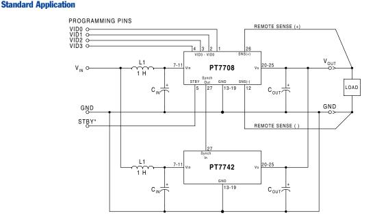
**External Capacitors:** The PT7742 requires a minimum ouput capacitance of 330µF for proper operation. The PT7742 also requires an input capacitance of 1500µF, which must be rated for a minimum of 1.4Arms of ripple current. For transient or dynamic load applications additional capacitance may be required. For more information refer to the application note regarding capacitor selection for this product.
